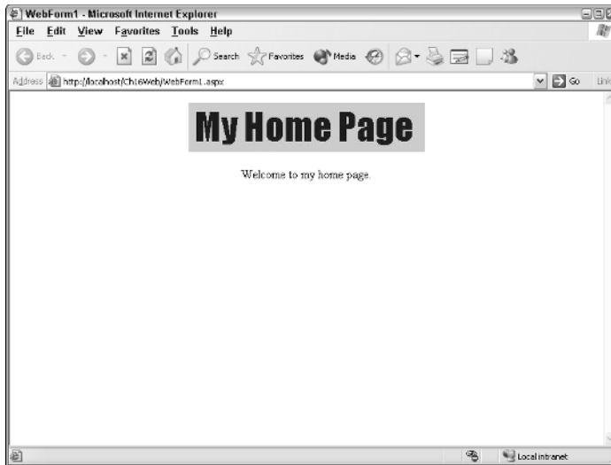
Figure 16.10 The browser output, showing the custom heading created by calling the RenderText method.
