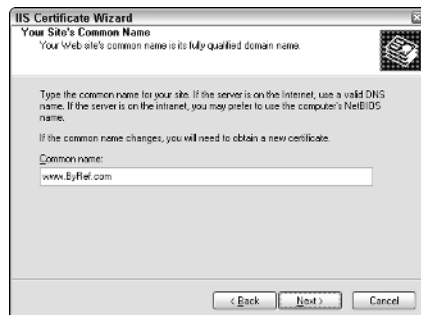
Figure 13.10 The common name must match the URL that is used when encrypted communication is required.
