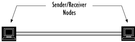
A point-to-point connection is direct.
